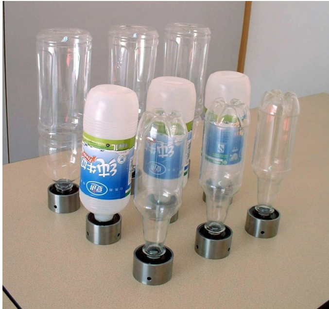
Figure 1. Finished Bottle Body Specimen for Water vapor permeability Testing
